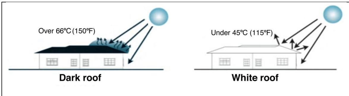
A few houses have flat concrete roofs that must be coated with a waterproofing product. White or a metallic reflective colour is preferable to darker colours for this product.
