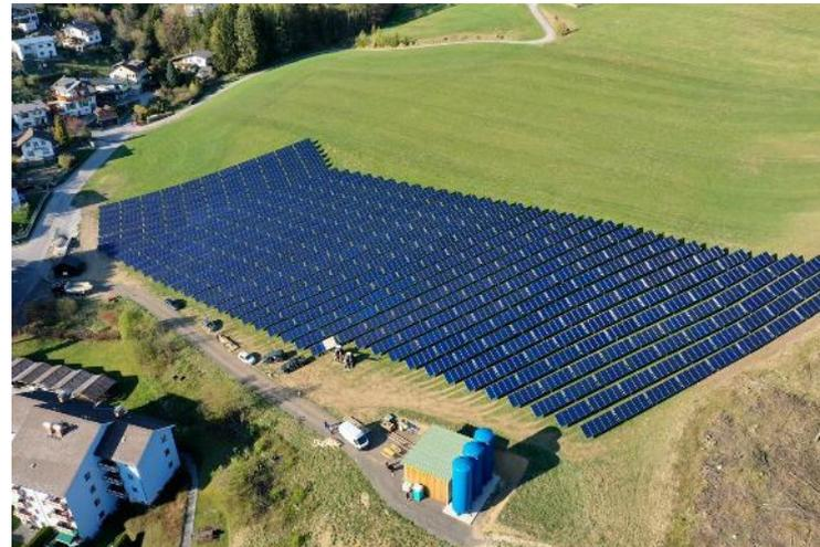
**Solar heat is fed into the flow of the district heating grid at up to 95°C.**
