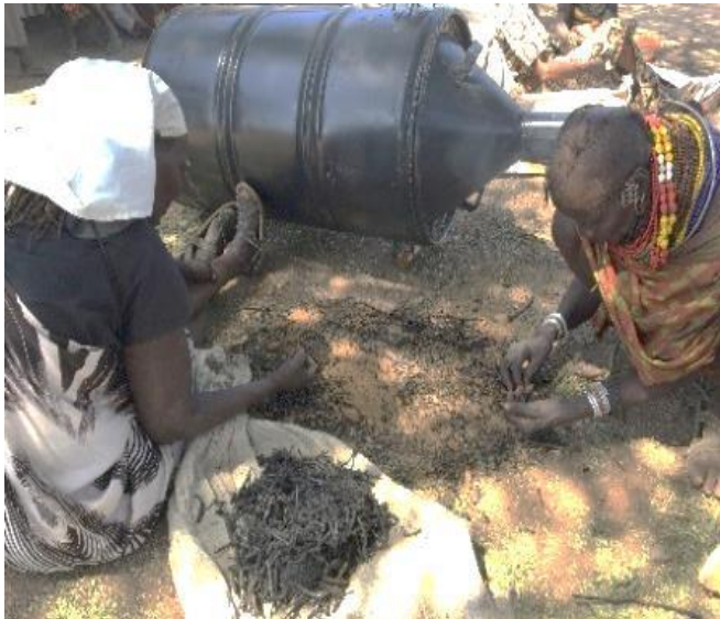
Charcoal production from twigs of invasive Prosopis juliflora using drum kiln Photo by Mary Njenga
