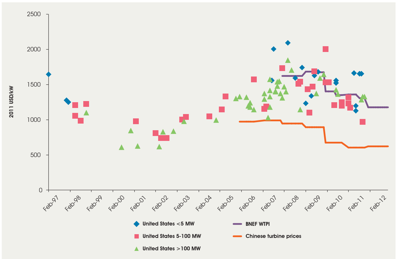
FIGURE 4.2: WIND TURBINE PRICES IN THE UNITED STATES AND CHINA COMPARED TO THE BNEF WIND TURBINE PRICE INDEX, 1997-2012
