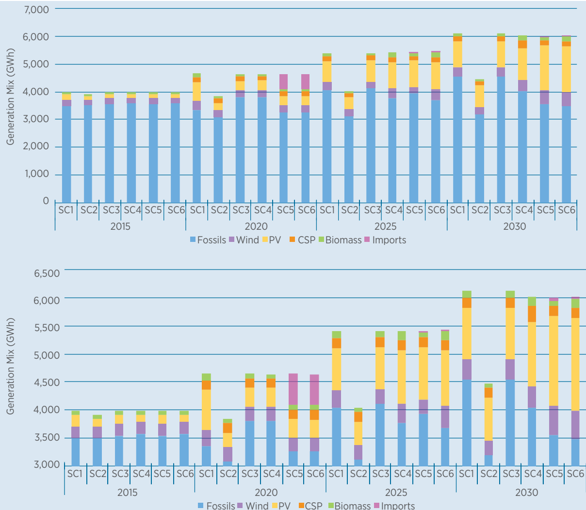
FIGURE 24: EVOLUTION OF GENERATION MIX IN THE SIX SCENARIOS. THE BOTTOM CHART PROVIDES A MORE FOCUSED OVERVIEW OF DIFFERENCES IN RENEWABLE ENERGY CONTRIBUTION IN DIFFERENT SCENARIOS (SELF-GENERATION FOR THE LNG TERMINAL IS EXCLUDED)
