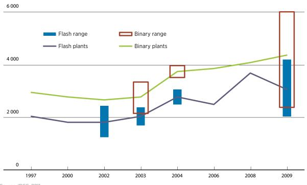
FIGURE 9.1: TOTAL INSTALLED COSTS FOR GEOTHERMAL POWER STATIONS, 1997 TO 2009 2014 USD/kW
