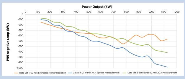
Figure 22: P99 of negative power output ramps for installed PV as a percentage of the available PV output
