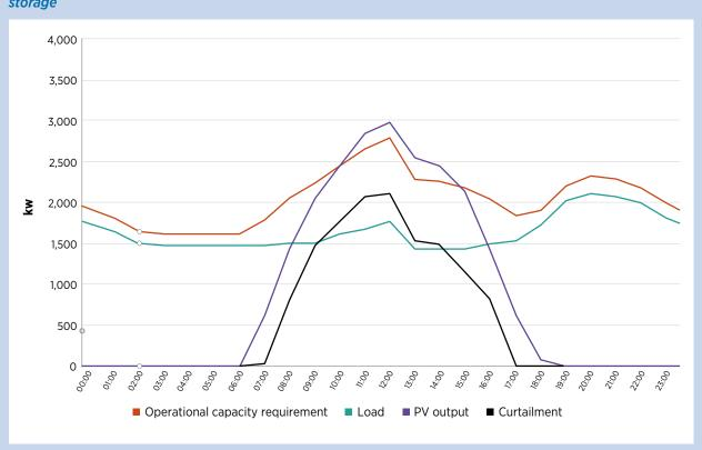
Figure 35: Impact on PV curtailment of additional 2.5 MWp of controllable PV (total PV 3.9 MW) without storage
