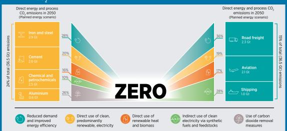
Figure 24 Emission reduction measures to reduce selected industry and transport CO<sub>2</sub> emissions to zero
