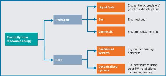
While power-to-heat is used for typical heating solutions in buildings and industry, power-to-hydrogen has more varied end-use cases, as seen below.
