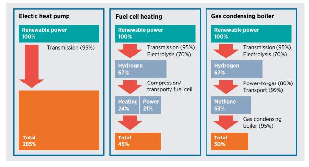
Figure 17 Efficiencies for different heating systems, starting from renewable electricity
