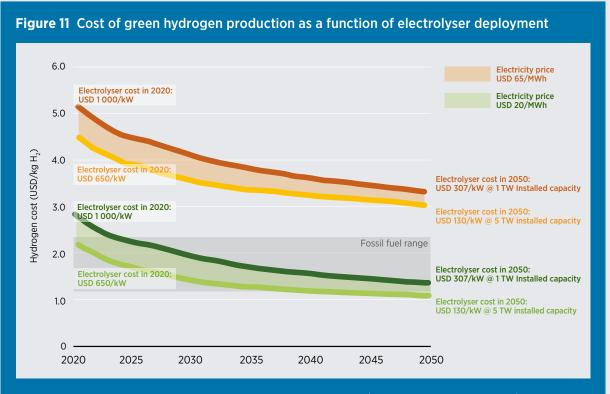
Note: Efficiency at nominal capacity is 65%, with a LHV of 51.2 kilowatt hour/kilogramme of hydrogen (kWh/kg H<sub>2</sub>) in 2020 and 76% (at an LHV of 43.8 kWh/kg H<sub>2</sub>) in 2050, a discount rate of 8% and a stack lifetime of 80 000 hours. The electrolyser investment cost for 2020 is USD 650-1000/kW. Electrolyser costs reach USD 130-307/kW as a result of 1-5 TW of capacity deployed by 2050. Source: IRENA (2020e).
